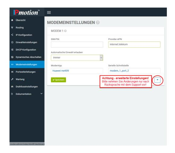
The menu for configuring the data modules allows changes to be made to the authentication for dialling in and the type of command transfer between the CAR-A-WAN.coach and the integrated data modules. All other fields not described in detail here may only be changed upon request by the IPmotion support and may cause a malfunction of the CAR-A-WAN.coach to the point of total failure.
