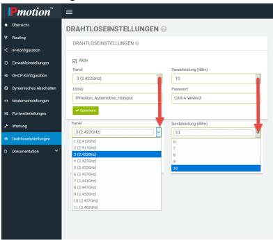
Here the optional access point for wireless LAN can be switched on or off, the network identification can be changed and the channel number can be set. The order also specifies the regulatory domain that restricts the available WLAN channels to the permitted channels and transmission powers.
