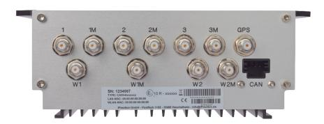
On the back of the device, in the upper row, you will find the connections for the mobile radio modems (WWAN 1-3) and their MIMO connections WWAN 1M-3M and GPS. The lower row contains the connectors for the WLAN antennas W1/W1M and the CAN connector.
