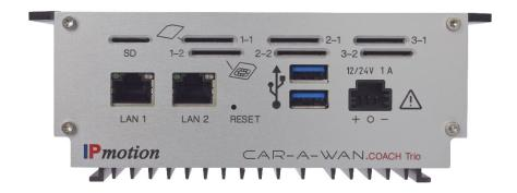
SIM 1 as default SIM card 1 in e.g. slot 1-1 with golden contact surface downwards until it clicks into place.
